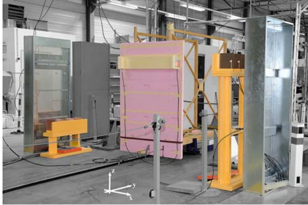
Fig. 7. Photograph of a gate setup with “free space” pallet and metal backplanes. The transmitter arrays are positioned on the stands to the left and right of the pallet mover, while the receiver antennas are mounted on the polyurethane foam slab. Note that the coordinate system is not at its origin.
